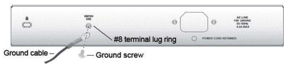
Figure 2.10 – Connect a Grounding Cable
