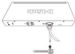
Figure 2-3. Slide the Retainer through the Tie Wrap
